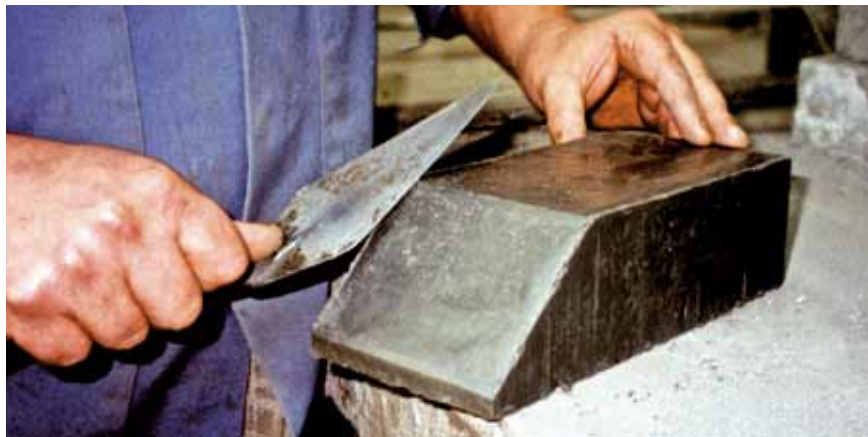
HAND FINISHED PLINTH HEADER
