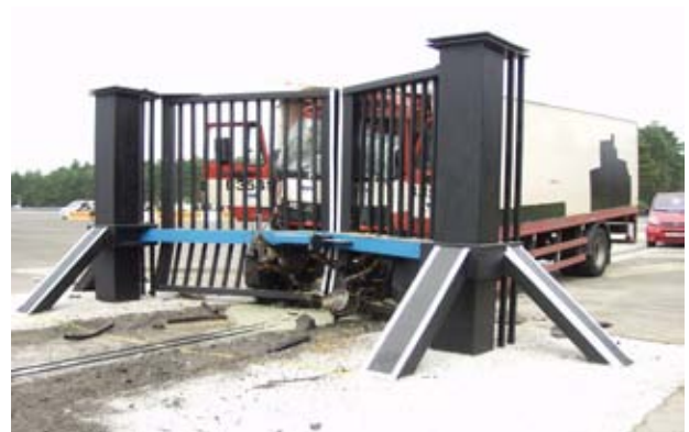
Fully functional post PAS 68 impact test
