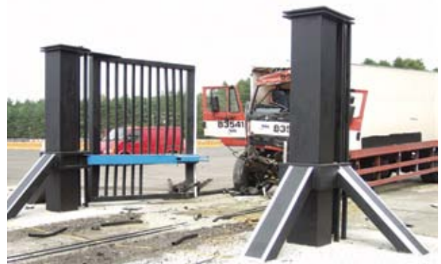
Fully functional post PAS 68 impact test
