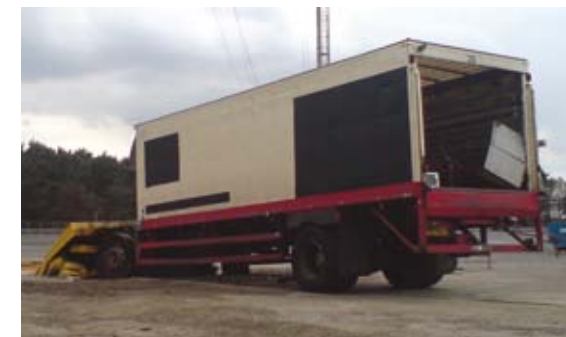
Terra Shallow Blocker post impact
