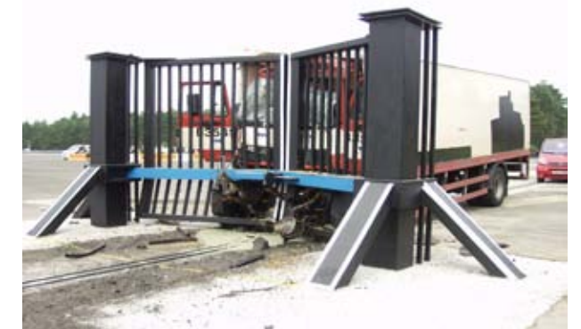
Fully functional post PAS 68 impact test
