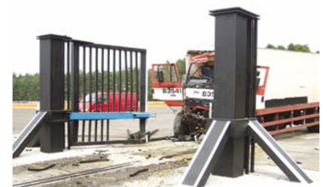
Fully functional post PAS 68 impact test
