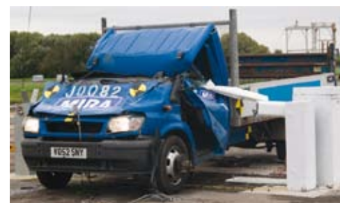
Compact Terra Barrier post impact test
