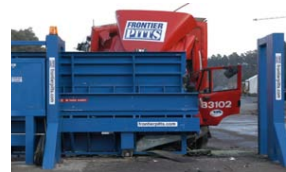
PAS 68 Terra Gate impact test in the half open position
