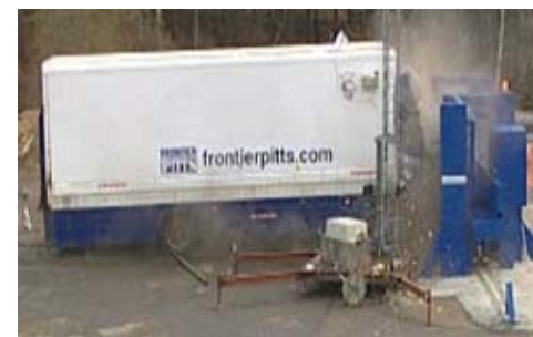
PAS 68 Terra Gate impact test in fully closed position
