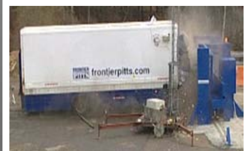
PAS 68 Terra Gate impact test in fully closed position
