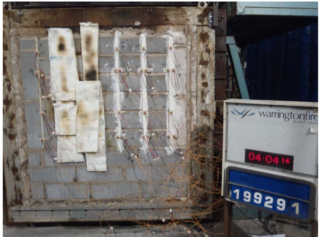
The unexposed face of the construction after a duration of 244 minutes
