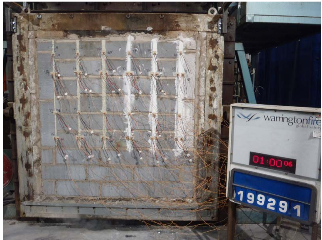
The unexposed face of the construction after a duration of 60 minutes
