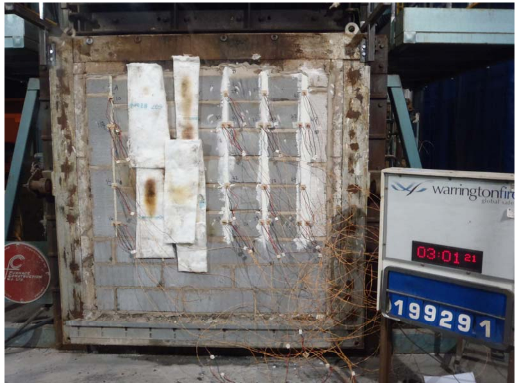
The unexposed face of the construction after a duration of 181 minutes
