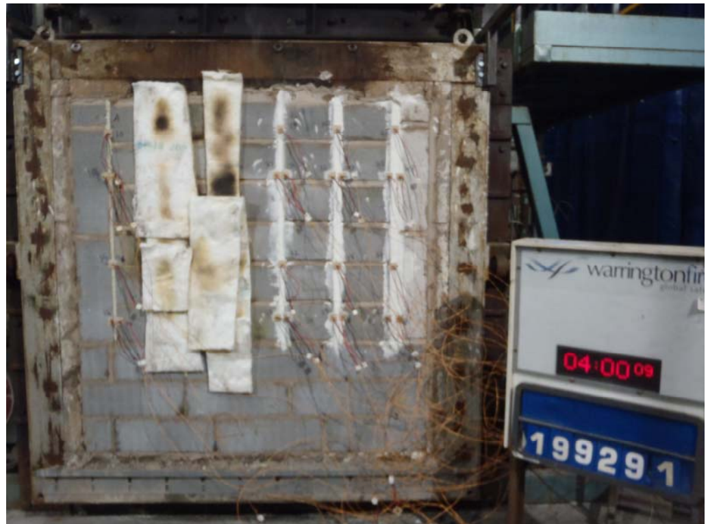
The unexposed face of the construction after a duration of 240 minutes
