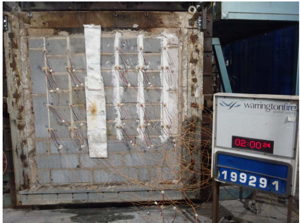
The unexposed face of the construction after a duration of 120 minutes
