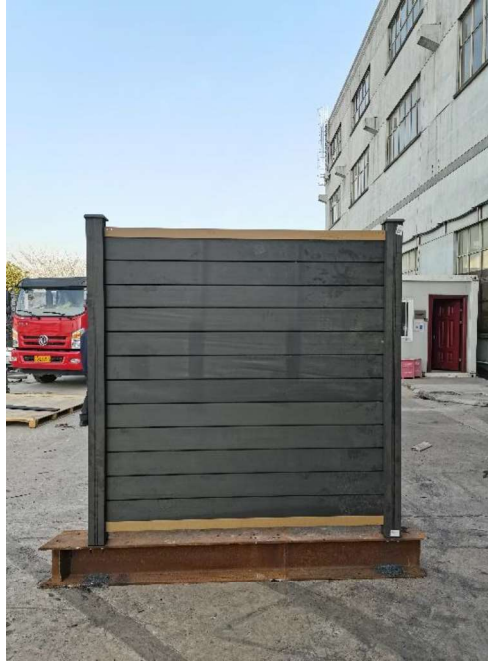
Photo No.1 Before Wind load Testing
