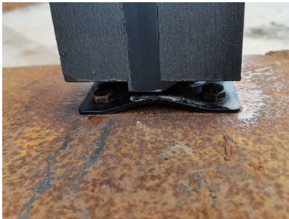
Photo No.3 After Wind load Testing at wind speed of 77 mph for 47 seconds
