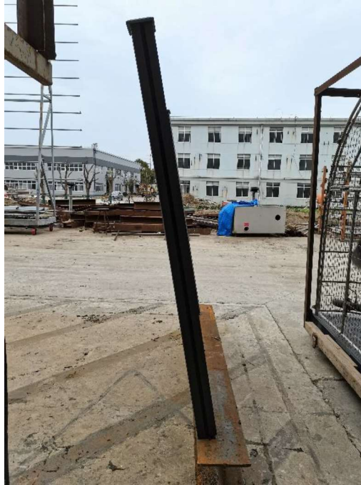
Photo No.3 After Wind load Testing at wind speed of 77 mph for 47 seconds
