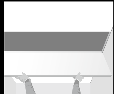
When being installed, the ceiling tile is pressed against the spring in the profile, clicking into the groove.
