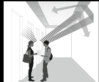
Ceiling sound absorption is particularly important beside the wall. In the angle between ceiling and wall, the ceiling surface is hit by direct sound and by sound reflected from the rest of the wall, so sound absorption is extra important.
