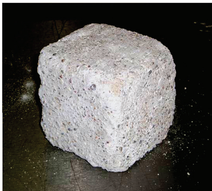
100% OPC Concrete showing more deterioration on exposure to silage effluent
