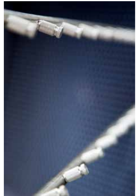
FIGURE 34-1: TOP HALF OF MANIFOLDS ANGLE DOWNWARDS, OTHER HALF ANGLE UPWARDS
