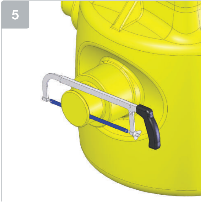
Saw off socket end/s, where inlet pipe/s are to be connected.
