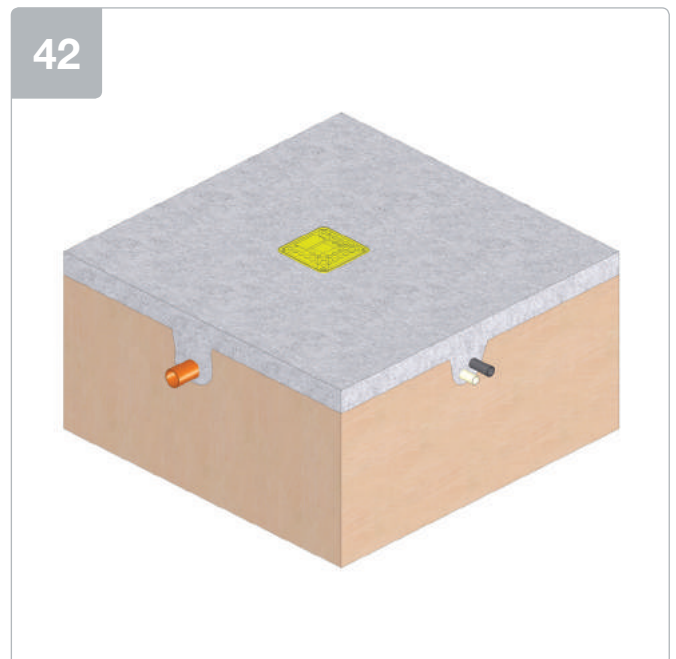
Re-fit temporary site cover to protect the pump station.
