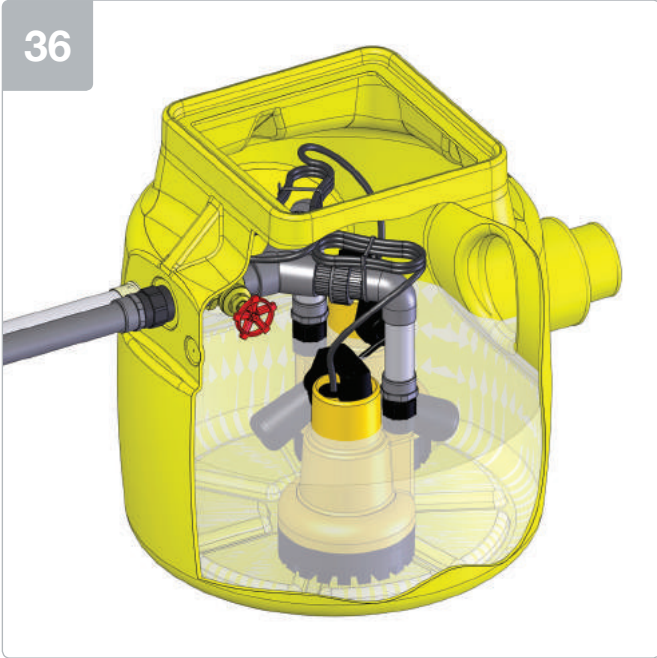
Lower pumps in to chamber. Ensure 'O' rings are correctly seated in unions and screw discharge arms to 'Y' piece manifold.
