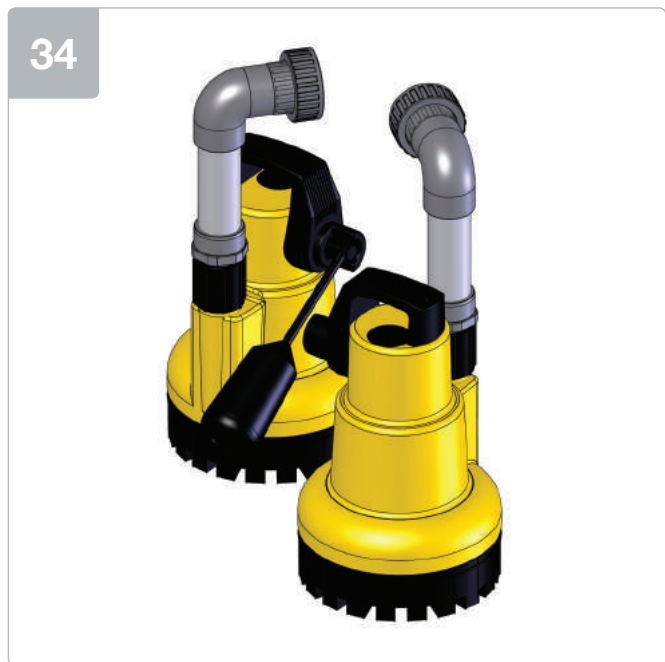
Wrap PTFE tape around thread located on male irons at the bottom of the discharge arms and screw discharge arms on to pumps.
