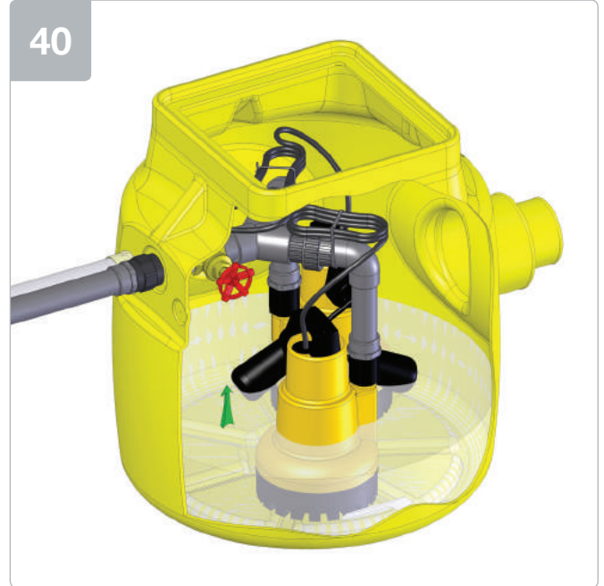
Turn mains supply on and lift each pumps float arm to test water is discharging correctly.
