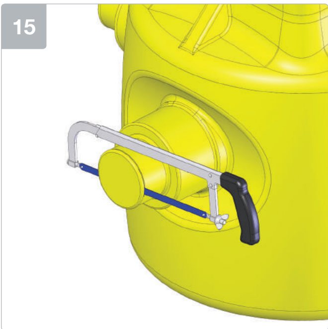
Saw off 110mm socket end/s to be used.
