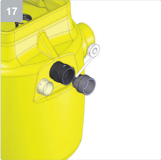
Wrap the thread on a DMS-0143 high pressure male iron with PTFE tape.
