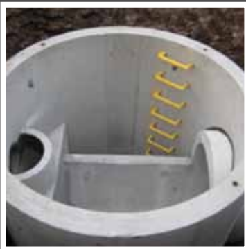
2100mm diameter wide wall manhole complete with pre-fitted ovoid butt and channel plus internal back-drop junction
