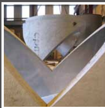
Side entry pipe and chamber section pre-cut ready for manufacture
