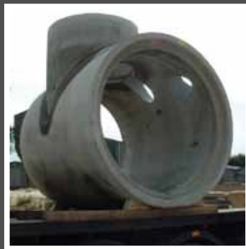
1800mm side entry manhole
