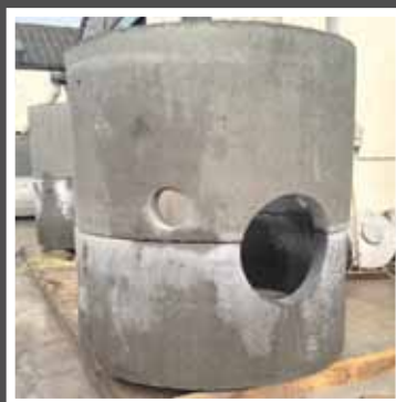
1200mm standard catchpit complete with cored holes over joint for a deep sump requirement
