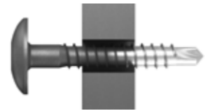
X : Fixing position hole diameter \varnothing 5 mm. When using Cembrit Facade Screw for Cembrit Cover, Cembrit Solid and Cembrit Transparent, you need to take off the washer before installation.
