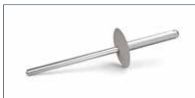
Cembrit Rivets Aluminium RIV-A EPDM Washer 4.0x20mm Aluminium body and Stainless steel mandrel. Unpainted or colour coated to the facade boards Grip Range 11-15mm
