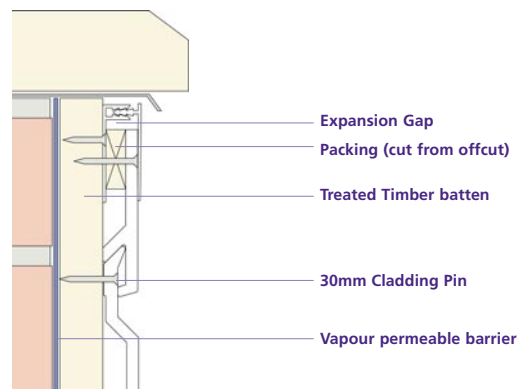
2-Part Top Edge Trim Installation to Window Cill
