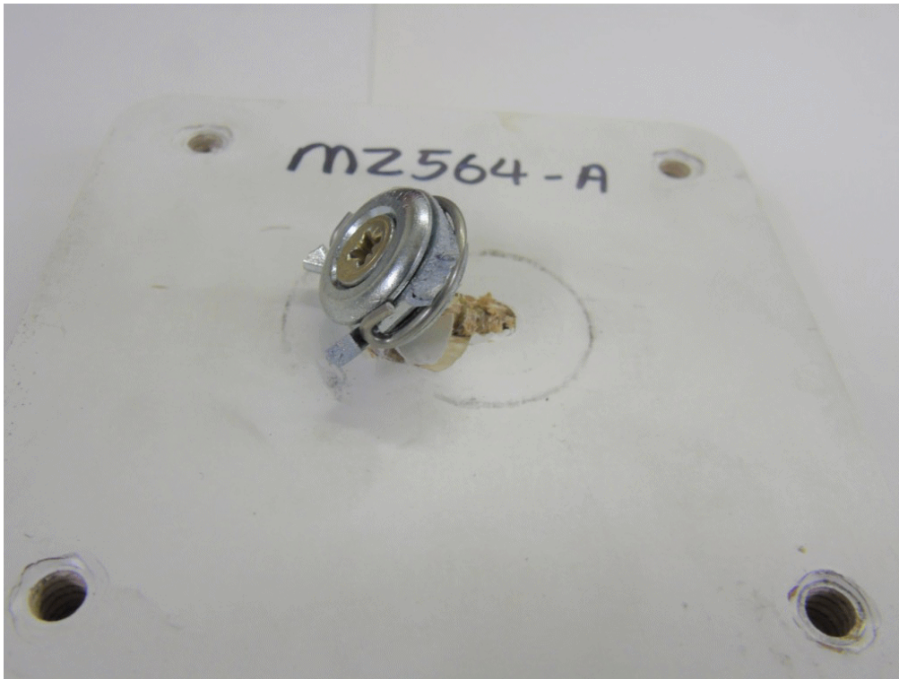
Photograph 1 A view showing the general condition of the button after a vertical shear test on a type 1 - metal fixing.
