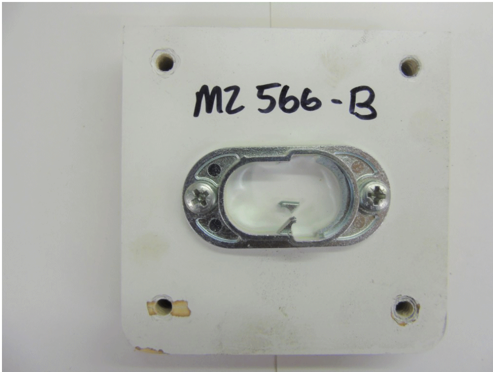
Photograph 5 A view showing the general condition of the fixing after a pull apart test on a type 1 - metal fixing.
