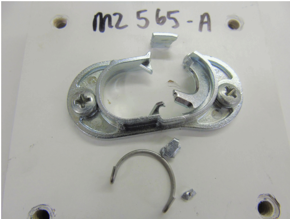
Photograph 3 A view showing the general condition of the fixing after a horizontal shear test on a type 1 - metal fixing.
