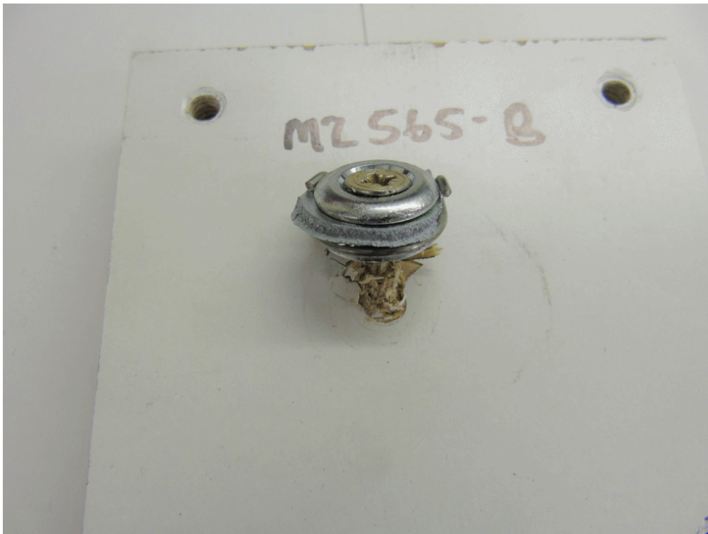
Photograph 4 A view showing the general condition of the button after a horizontal shear test on a type 1 - metal fixing.
