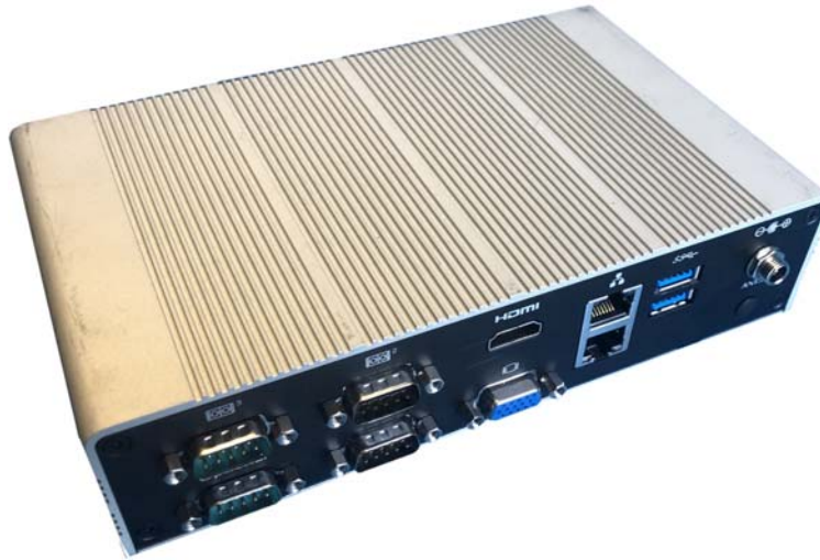
Figure 1.5 — Typical Embedded PC
