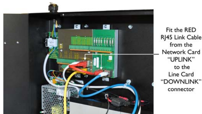
Figure 2.23 — Red RJ45 Link Between Network and Line Card
