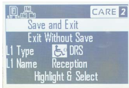
Figure 4.19 — Save and Exit Outstation 1 Parameters
