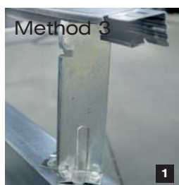
1. Fix the Ashgrid ABV Brackets to the structure, with the mouth of the ABV facing downslope, ensuring that the brackets are in line (it may be useful to use an AG40 bar to align the brackets)
