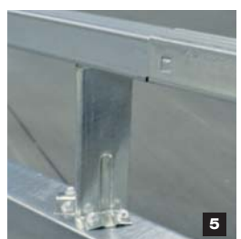
4/5. Once the Ashgrid bar is in place, the next bar may then be connected to it, by locating the open end onto the 'Safe-Loc' spigot and pushing firmly until the tab clicks into position. This bar may then be snapped onto the brackets as before
