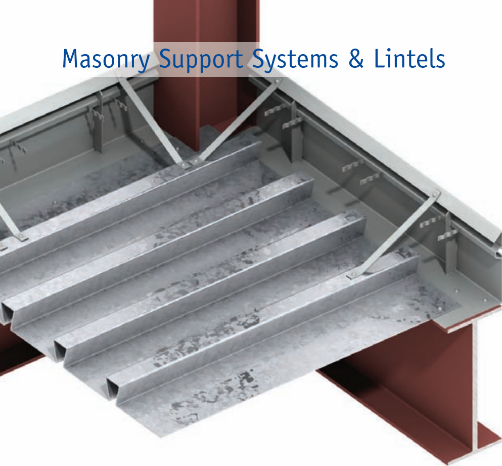
Corner Detail Showing Fixing Straps Between CombiDeck and Metal Deck Shuttering
