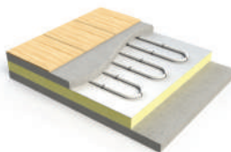
Pipe into Screed
