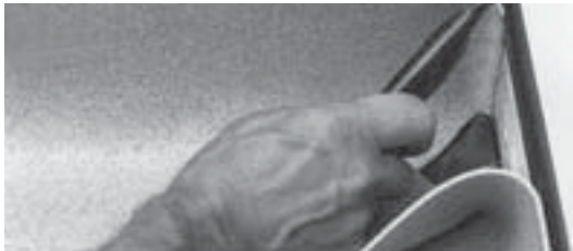
3. Fold in one side of the mitre and carefully cut off the surplus material.
