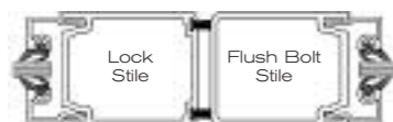
Section showing relationship between the Lock and Flush Bolt stile for the ACS 10D
