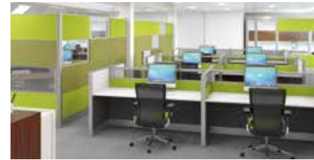
3. Screens of STC or R_w of at least 18 dB and NRC or \alpha_w of at least 0.7 to a minimum height of 500 mm above desk level (preferably floor standing screens exceeding 1500 mm) between all work stations, including side-by-side.
