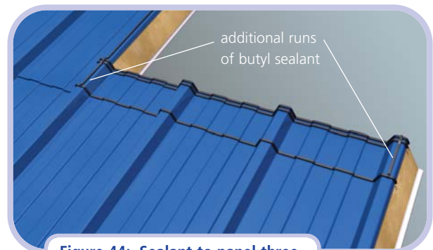
Figure 44: Sealant to panel three
