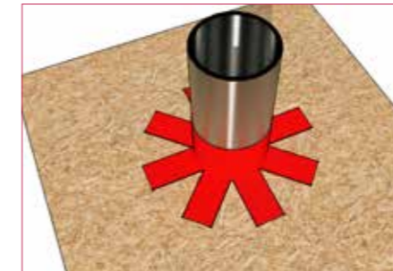
Firmly press tape to substrate
