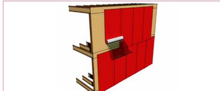
Diagram showing staggered lap of vertical installation of Wraptite-SA
