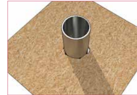
Pipe penetration with airgaps around pipe
