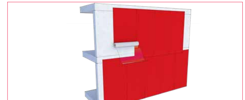
Fig.3 Staggered vertical installation of Wraptite membrane.
