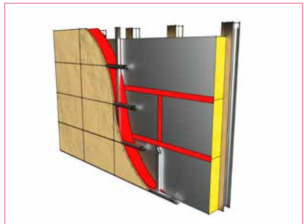
Seal joints of rigid insulation with Wraptite tape / or use Wraptite
