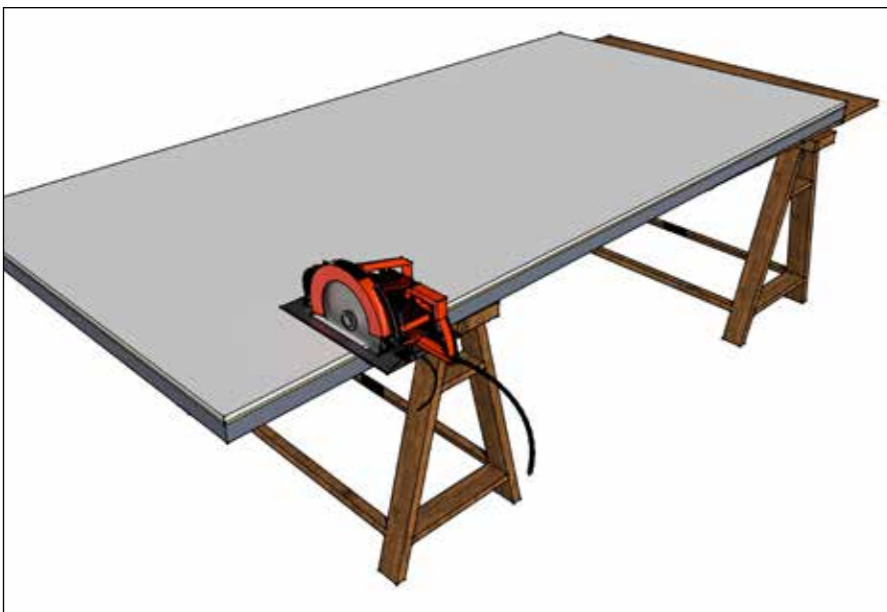
Fig. 2 Cutting Spacetherm WL boards
