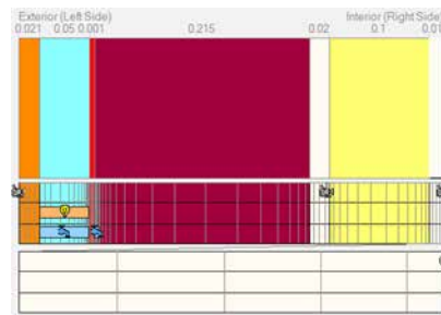
Rainscreen Brick Wall with internal PIR /Rockwool
