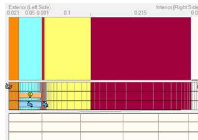
Rainscreen Brick Wall with external PIR/Rockwool
